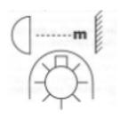
The symbol wich appears on somes lamps indicate the mandatory use of a bulb, be sure that the above symbol appears on the packaging of the new bulb.
